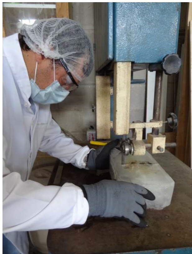
Figure 2. Saw used to cut the block of ice.
