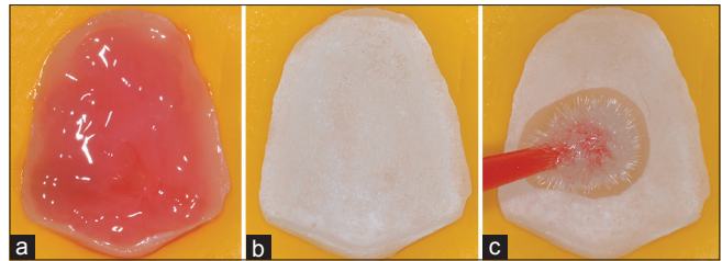
Figure 4: (a) 9.6% hydrofluoric acid applied in the inner surface of the ceramic. (b) Inner ceramic surface after rising the hydrofluoric acid gel with water and dried. (c) Silane-coupling agent application
