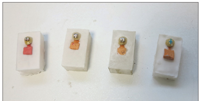
Figure 1: Crowns on their respective dies embedded in acrylic blocks
