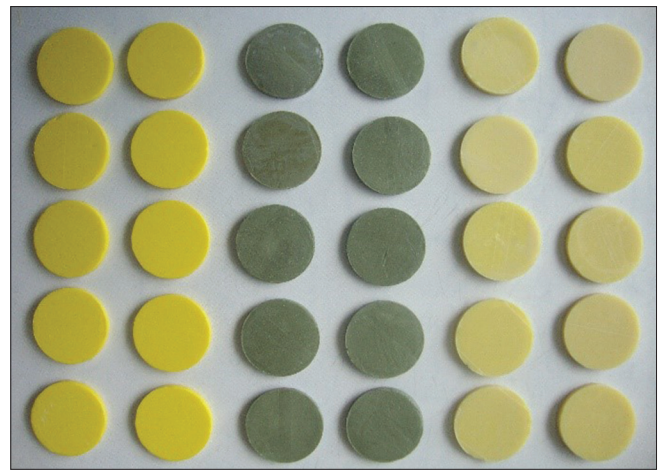
Figure 6: Test samples. Silicone (yellow), Aluwax (grayish green) and polyether (light yellow)
