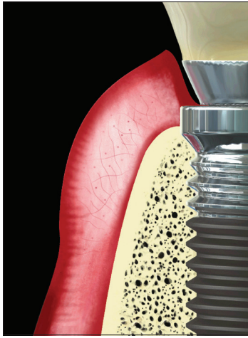
Figure 2: Schematics of a platform switching system and surrounding hard and soft tissue profile
