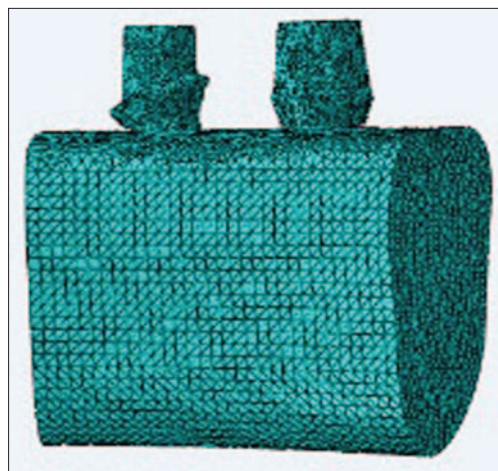
Figure 2: 15° angulated premolar implant and molar straight implant
