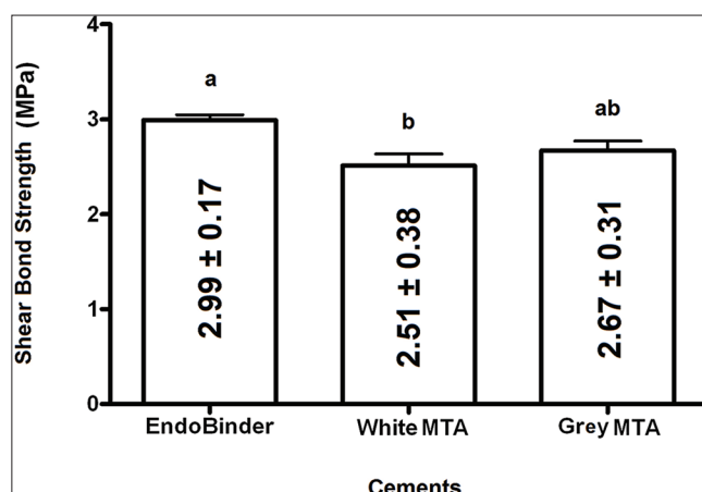
Figure 3: Graphic representation of the mean values (MPa) and standard deviations of the shear bond strength test ( n = 20 ). Different lowercase letters over columns indicate statistically significant difference. Tukey's test categories with the same letter are not statistically different from each other ( P < 0.05 ) 1-way ANOVA and Tukey's tests, P < 0.05 P = 0.0803
