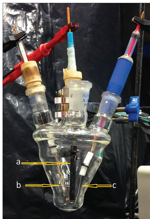
Figure 1: Schematic diagram of electrically activation of sodium hypochlorite; (a) working electrode (pyrolytic graphite electrode), (b) auxiliary electrode (platinum sheet), (c) reference electrode (Ag/AgCl)
