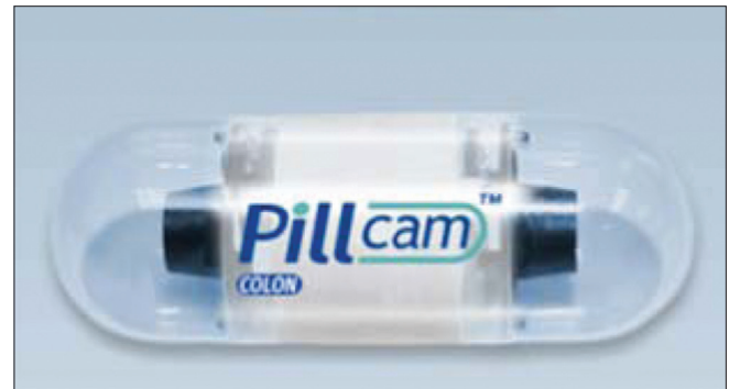
Figure 2: Colon capsule with two video cameras, one at each end of the capsule
