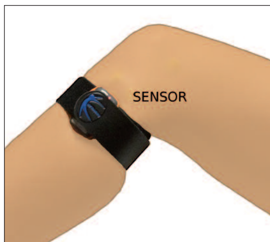
Fig. 2. Acceleration sensor set-up: the sensor was positioned between the lateral aspect of the anterior tuberosity and Gerdy's tubercle.
