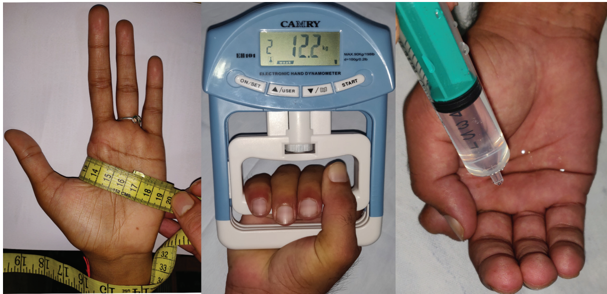
Fig. 1 This figure shows a few methods of measurement used in the methodology of the study. On the left side, the figure shows the measuring of the palmar circumference with the standard measuring tape. In the center, grip strength is measured with the hand dynamometer. On the right, palmar volume is being measured with the cupping of the hand and holding as much water as possible.
