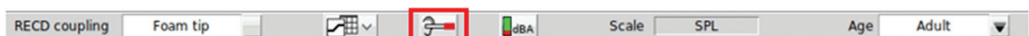
Figure 2 Probe guide button. Note that "adult" must be selected under the Age dropdown menu to use this feature. The feature was developed using data from a variety of adult ears, 5 which cannot be generalized to pediatric ears.
