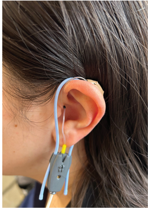
Figure 12 Probe tube and RITE in an ear.
