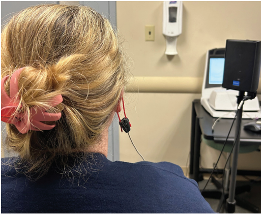
Figure 18 Setup for CROS verification (probe microphone still in left ear only, reference microphone on right side, speaker at 45 degrees).
