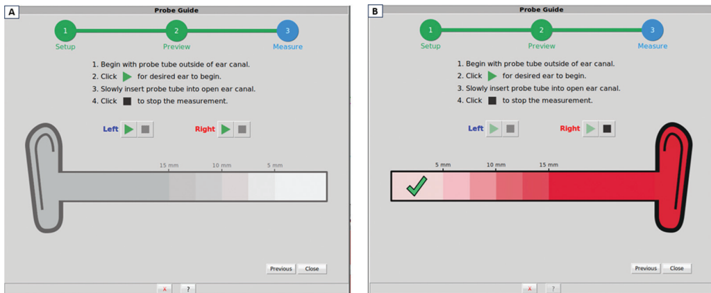
Figure 3 Probe guide process. (A) Probe guide setup screen; (B) successful placement of probe microphone.
