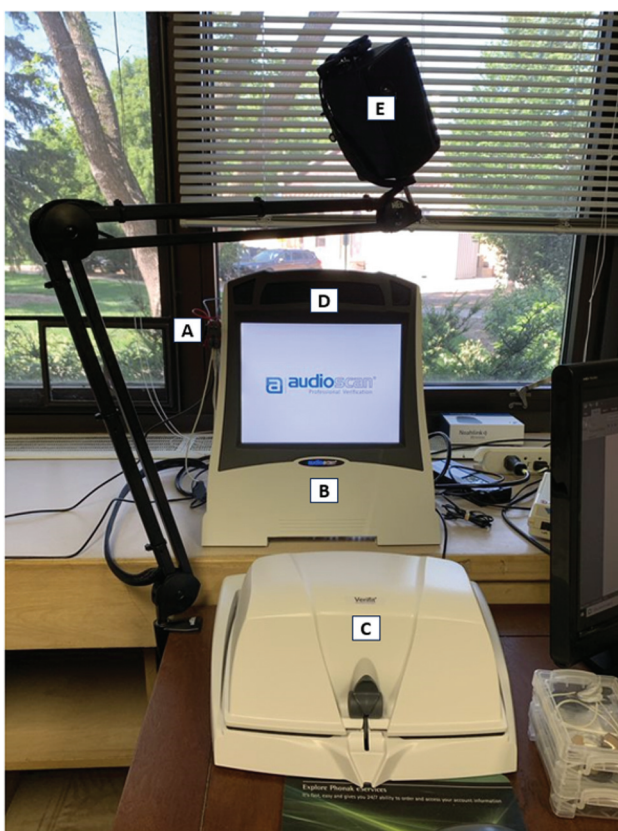
Figure 1 Audioscan Verifit 2 probe microphone and test box equipment. (A) Probe microphones (in dock); (B) display unit; (C) test box; (D) internal speaker; (E) external speaker.
