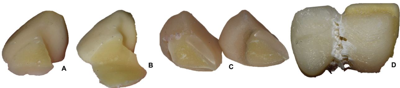
Fig. 6 Details of fractured resin-bonded bridges (RBBs) and more frequent failure modes by material type. (A) ENA, adhesive interproximal and cohesive in retainer. (B) Y-ZPT, adhesive, with RBB integrity. (C) SUP, cohesive in Frasco tooth and retainer. (D) ABS, adhesive in interproximal, cohesive with plastic deformation in RBB (no RBB tooth loss occurred).
