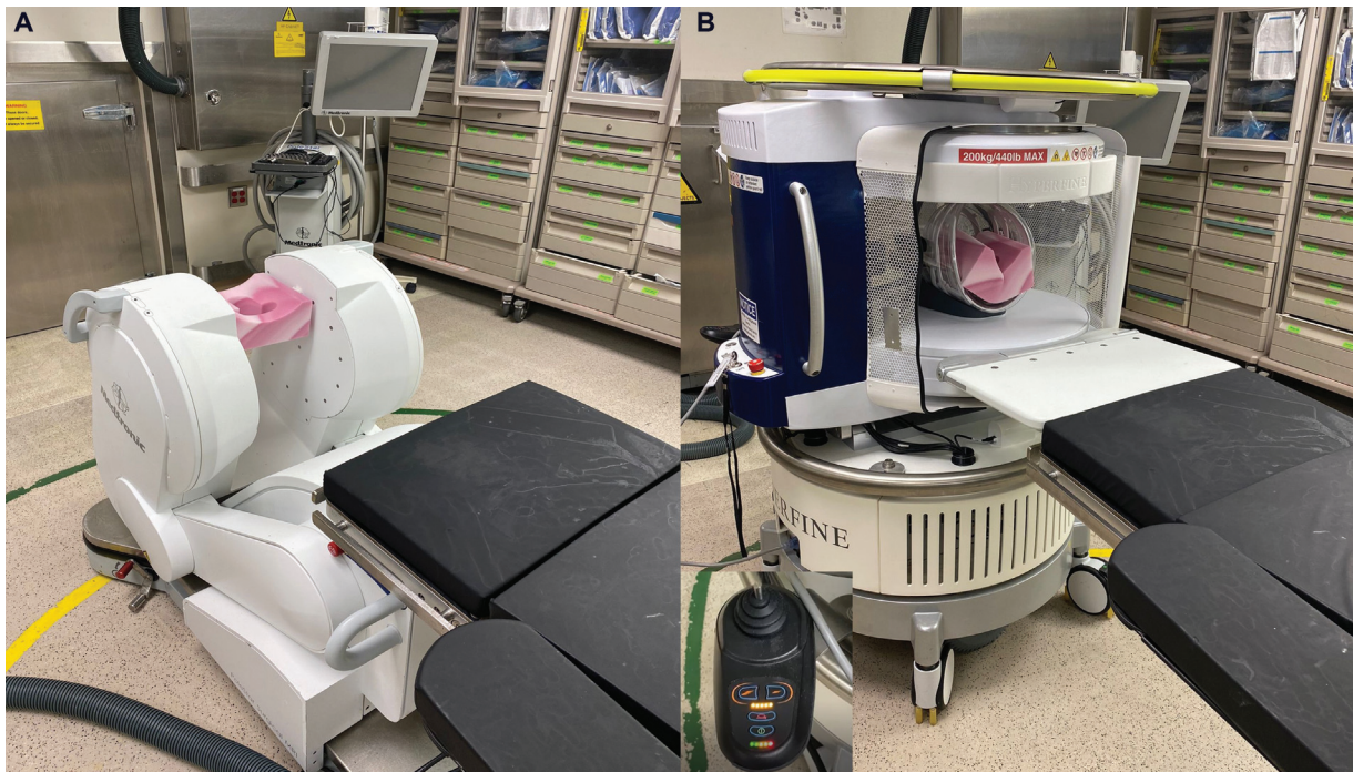
Fig. 1 (A) Medtronic (0.15 T) scanner. (B) Hyperfine (0.064 T) scanner. Pictured in the bottom left is the joystick that enables easy maneuverability.
