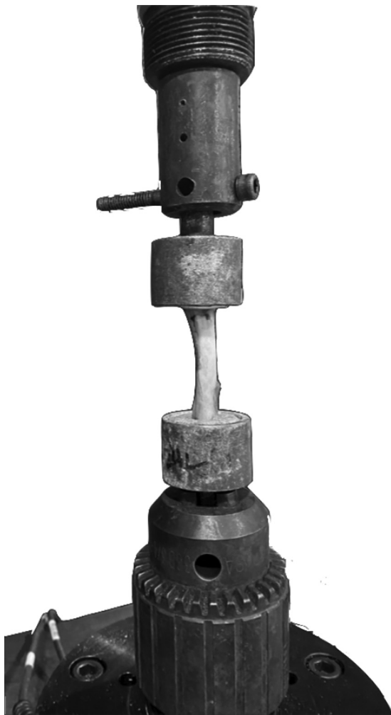
Fig. 2 Photograph of the mechanical testing setup with the embedded specimen attached to the load cell (bottom) and biaxial material testing machine (top).
