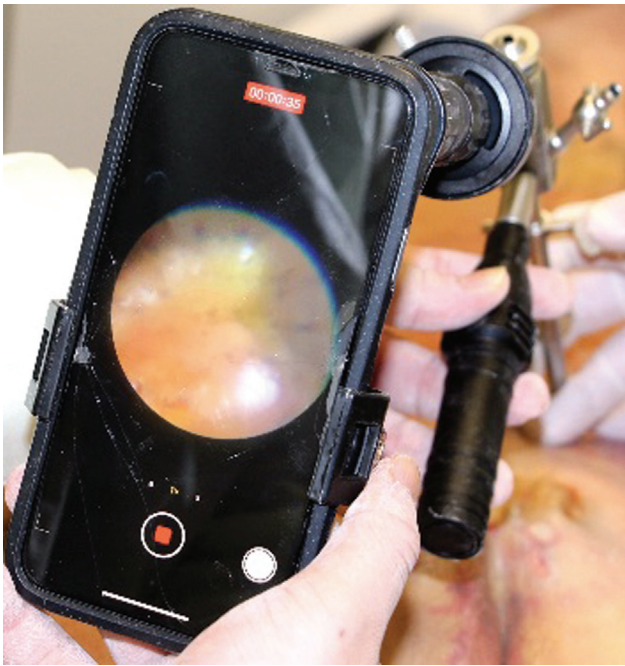
Fig. 1 Optical smartphone camera adapter attached to the endoscope in addition to a portable LED lamp.
