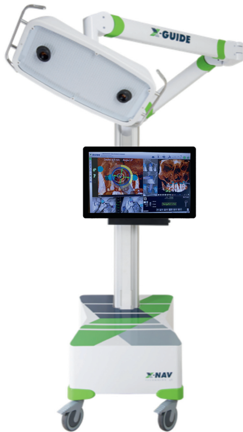
Fig. 1 Dynamic navigation system (DNS) console.
