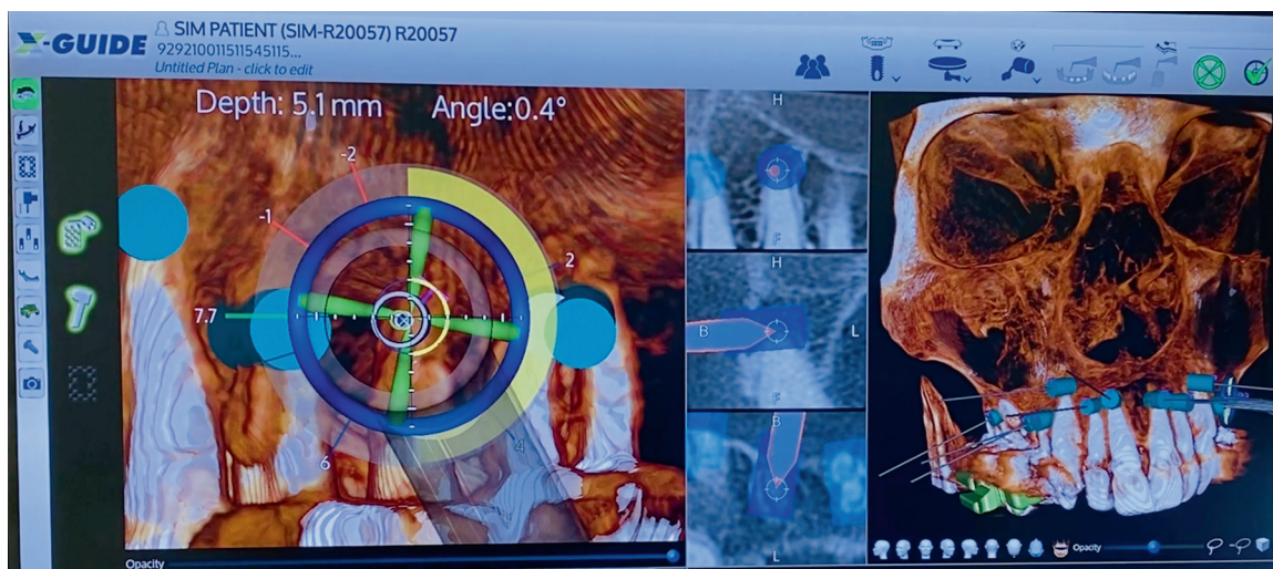
Fig. 3 Surface of the dynamic navigation system (DNS) during endodontic microsurgery.
