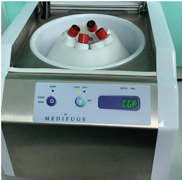
Fig. 1 Medifuge MF200 (Silfradent, Italy) with specific program at 30 seconds for acceleration, 2,700 rpm for 2 minutes, 2,400 rpm for 4 minutes, 2,700 rpm for 4 minutes, 3,000 rpm for 3 minutes, and finally with deceleration for 36 seconds.
