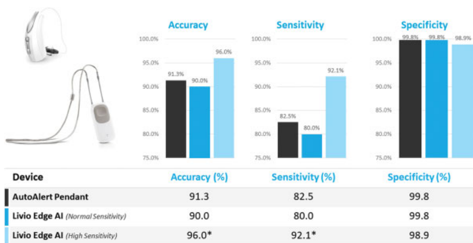
Figure 11 Measured fall detection and alert accuracy \{[(\text{true positives} + \text{true negatives})/\text{total trials}] \times 100\} , sensitivity \{[\text{true positives}/(\text{true positives} + \text{false negatives})] \times 100\} , and specificity \{[\text{true positives}/(\text{true positives} + \text{false negatives})] \times 100\} for a popular neck-worn pendant (AutoAlert) versus Livio Edge AI with normal and high sensitivity. Accuracy, sensitivity, and specificity were compared across the three fall detection systems with McNemar's test for paired nominal data. Livio AI (normal sensitivity) was more accurate than AutoAlert [ \chi^2(1) = 9.13 , p = 0.002 ] and Livio AI (high sensitivity) [ \chi^2(1) = 27.03 , p < 0.001 ]; the difference in accuracy between Livio AI (high sensitivity) and AutoAlert was not significant [ \chi^2(1) = 0.36 , p = 0.550 ]. Livio AI (normal sensitivity) was significantly more sensitive than AutoAlert [ \chi^2(1) = 9.98 , p = 0.002 ] and Livio AI (high sensitivity) [ \chi^2(1) = 29.00 , p < 0.001 ]; the difference in sensitivity between Livio AI (high sensitivity) and AutoAlert was not significant [ \chi^2(1) = 0.51 , p = 0.47 ]. Livio AI (high sensitivity) was significantly more specific than Livio AI (normal sensitivity) [ \chi^2(1) = 4.00 , p = 0.045 ]. However, specificity differences were not statistically significant between Livio AI (normal sensitivity) and AutoAlert [ \chi^2(1) = 3.57 , p = 0.059 ] or between Livio AI (high sensitivity) and AutoAlert [ \chi^2(1) = 1.00 , p = 0.317 ]. 4
