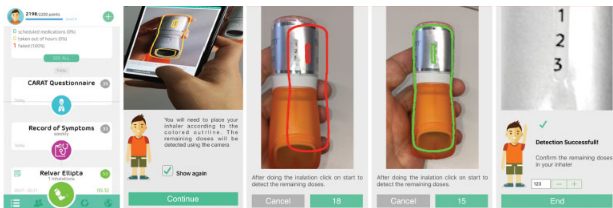
Fig. 5 Workflow for dosage detection counter.
