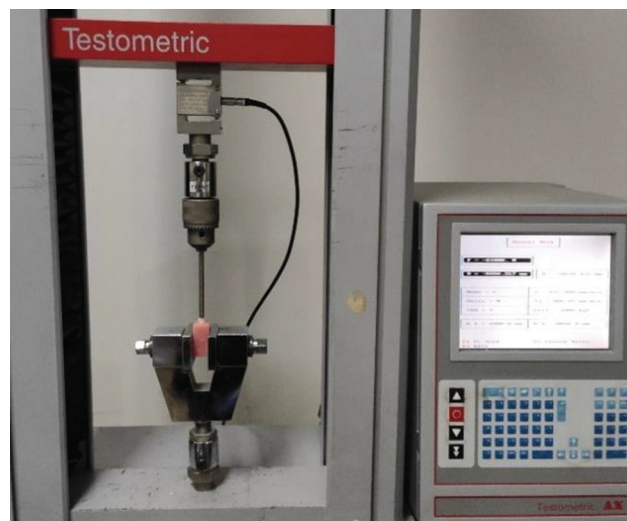
Fig. 3 Universal mechanical testing machine (Testometric).
