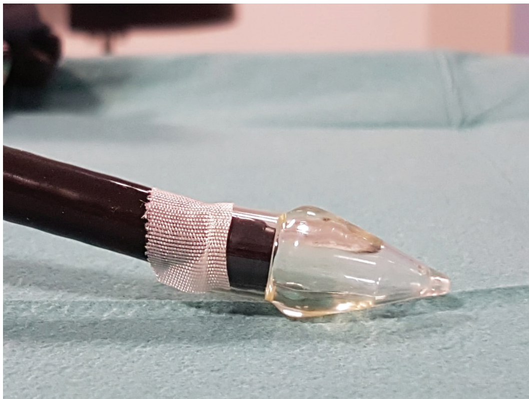
Fig. 2 The BougieCap device slipped on and being taped to the end of an upper endoscope.
