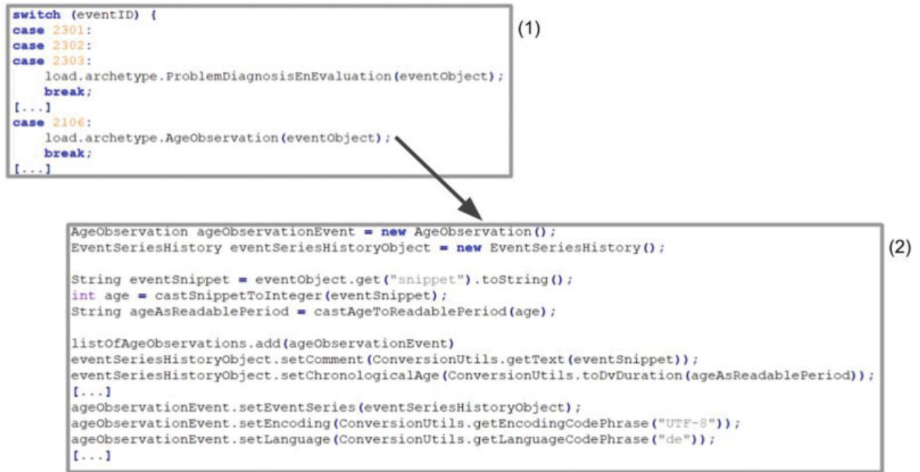
Fig. 3 Snippet from the Java code for mapping the extracted information snippet on unique archetype paths (mapping and integration module), including (1) running through all defined rules and the firing of a suitable rule which then (2) enables the instantiation of a new age observation by filling the associated archetype paths with the extracted information delivered in the eventObject.
