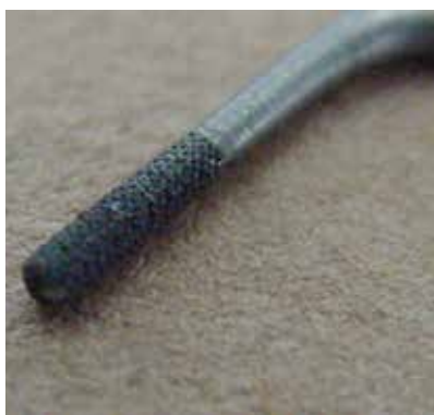
Figure 1a. Diamond coated CVD bur.
