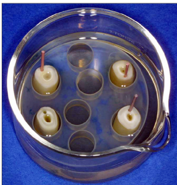
Figure 1. Experiments were carried out in glas jars filled with sterile anaerobic NaCl/serum medium and containing the medicated and non-medicated root specimens as well as the bacterial growth controls.
