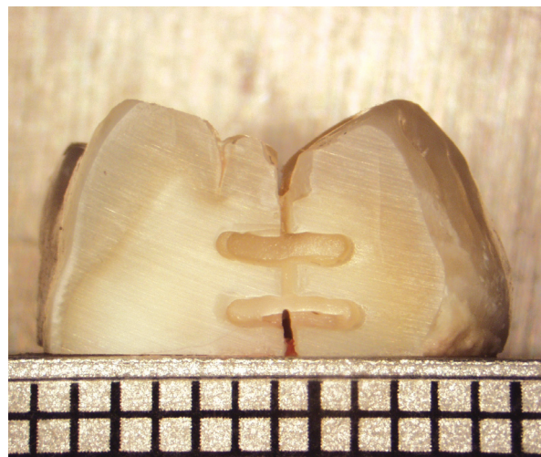
Figure 1. Specimen cut horizontally at the dentino-enamel junction to remove the roots, with one of two flattened axial surfaces visible, showing fine vertical groove to direct splitting, and two horizontal orientation notches. Grid lines represent 1mm.
