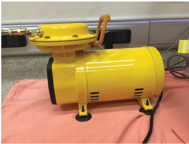
Fig. 7 Air compressor for particle dispersion.
