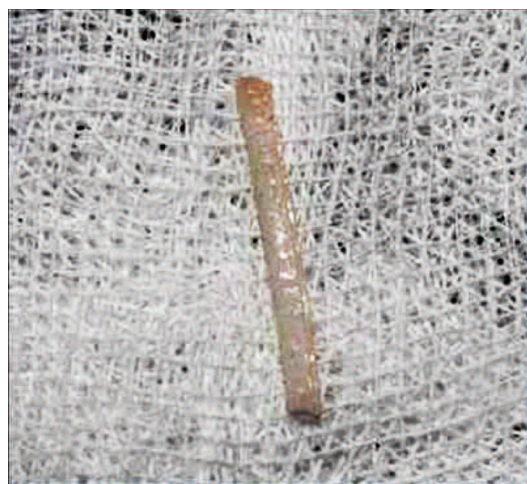
Fig. 3 3D printed polymeric scaffold (Cubex).
