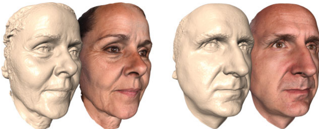
Fig. 5 Visualizations of computerized 3D models of the face, high-resolution geometry and photographic texture acquired with our stereophotogrammetric setup.
