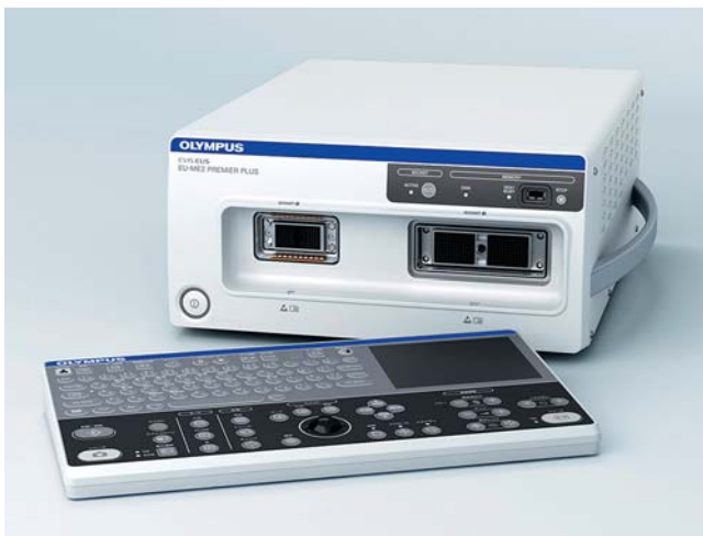
Fig. 1 The EU-ME2 is a high-quality compact ultrasound processor for use with endoscopic ultrasound equipment that has been designed for integration with conventional endoscopy on a single workstation. It is possible to use new functions such as Tissue Harmonic Echo (THE), Contrast Harmonic EUS (CH-EUS) and Elastography.
