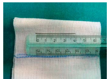
Fig. 3 Image of the removed fractured needle fragment, which measured 4 cm in length.
