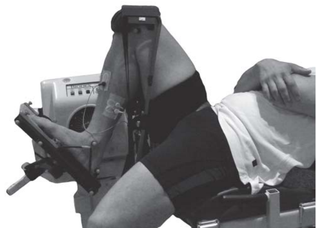
Fig. 1 Setup for maximal mechanical power measurement during plantar flexion. Measurements were performed with knees bent to minimise the effect of gastrocnemius muscle and selectively determine the power of the soleus muscle.
