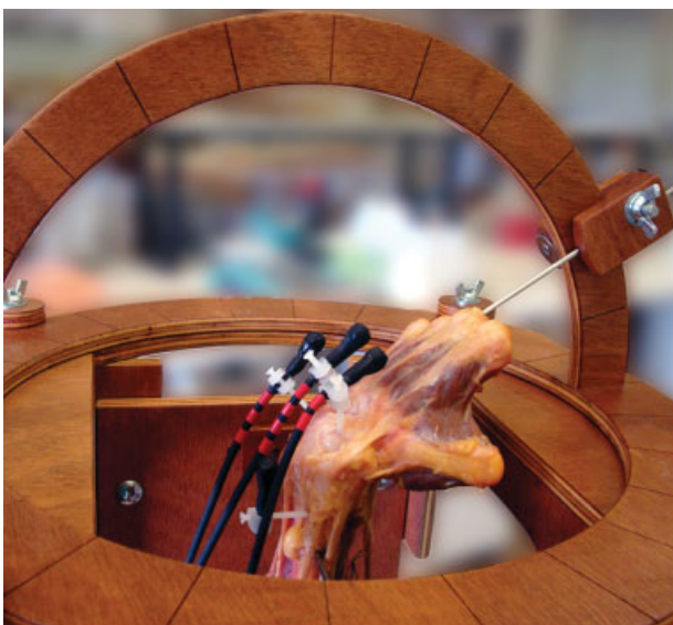
Fig. 8 Photograph of a specimen set in a specially designed jig to investigate the effect of individual muscle contraction in the alignment of the carpal bones. Black sensors are attached to specific bones to assess three dimensional carpal rotations. (URBES laboratory, Department of Anatomy, Universitat de Barcelona, Spain.)
