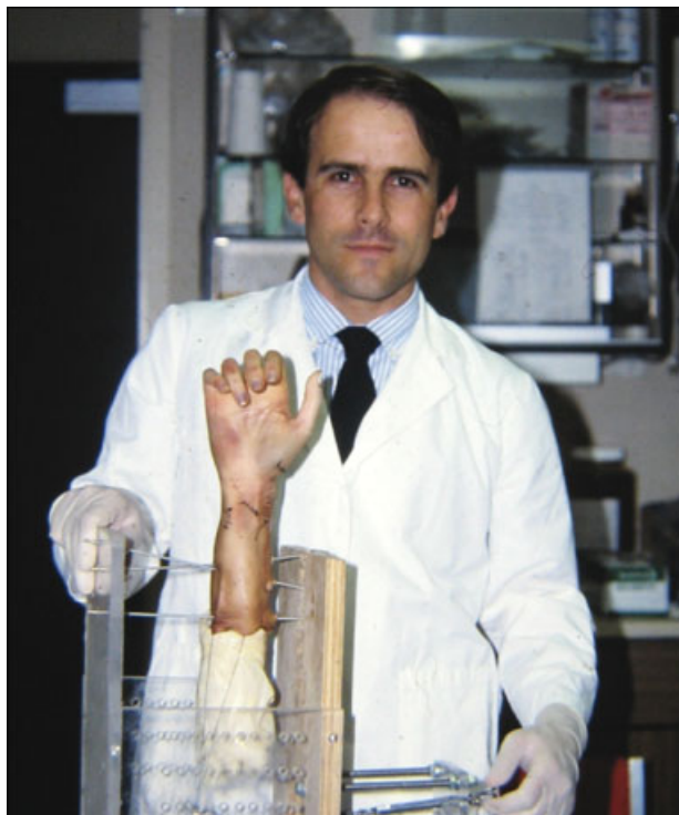
Fig. 1 Preparing a specimen to investigate the effects of partial carpal fusions in the kinematics of the wrist. Biomechanics Laboratory, Mayo Clinic, Rochester MN. October 1987.
