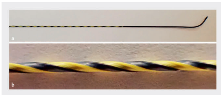
► Fig. 2 The novel guidewire measures 0.035 inches and features a thick, high-rigidity nickel-titanium core. The surface is coated with polytetrafluoroethylene, using “ridge-processing”, which reduces contact area and friction with devices, enhancing followability and insertability.
