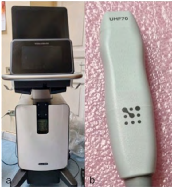
► Fig. 3 Ultrasound scanner with three ultra-high-frequency probes (25–48–70-MHz) by Vevo MD, Fujifilm Visual Sonics (a). Linear probe of 70 MHz (b).
