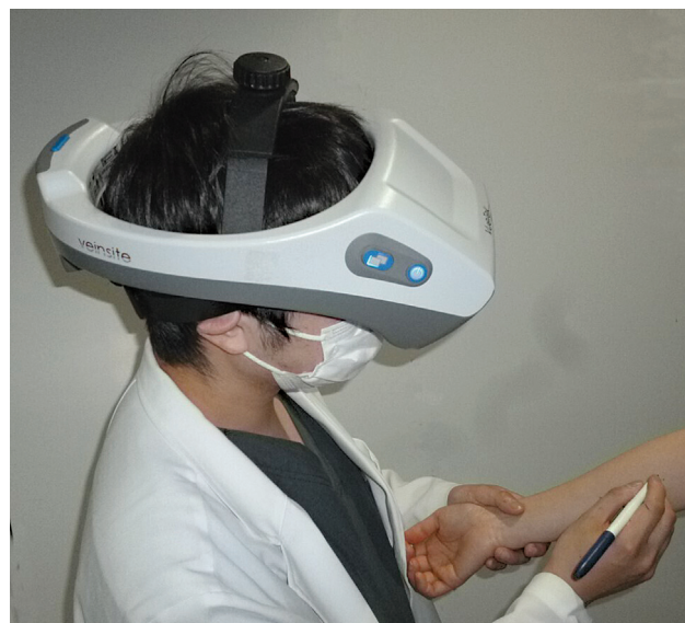
Fig. 1 Veinsite is a high performing, non-contact, vein viewer. Adjust it with the upper and posterior notches until the appropriate position is met. When you wear the device on your head, you will be able to see the screen inside the main unit. The screen shows a visualized image of blood vessels.
