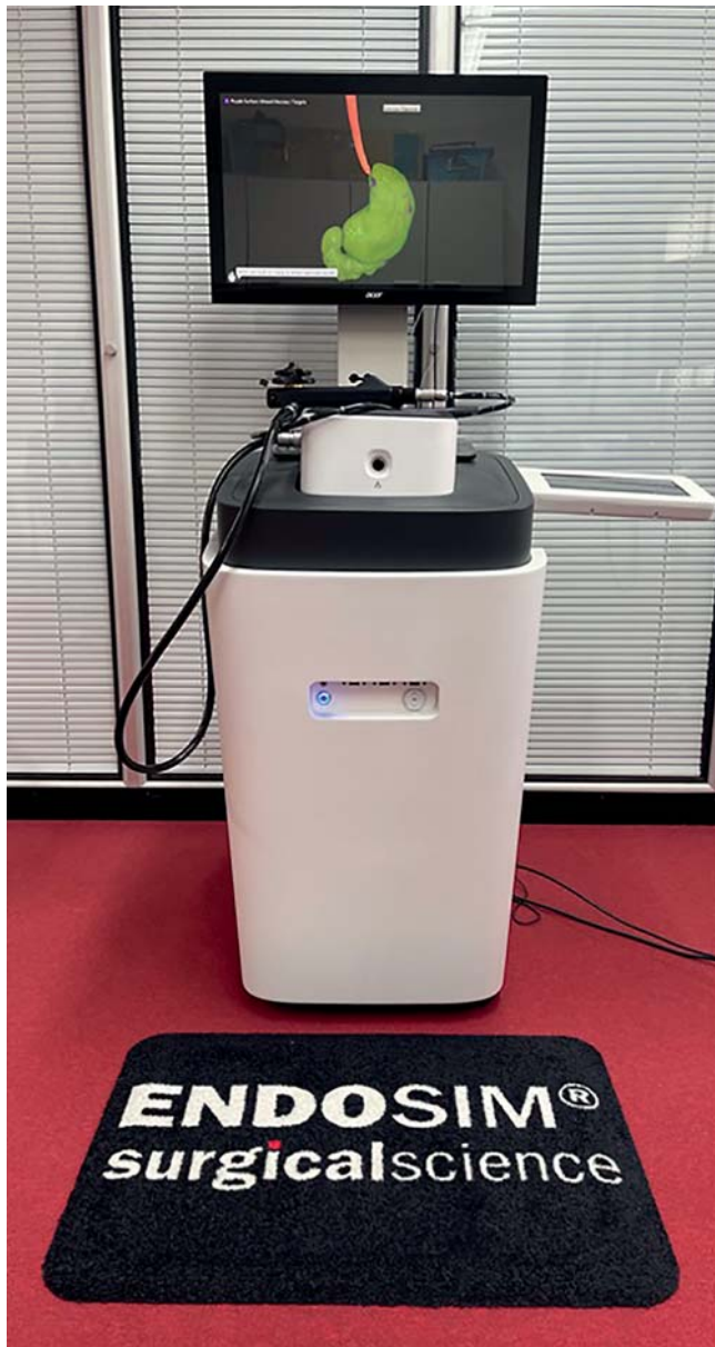
► Fig. 1 A Simcart, table-mounted, height-adjustable EndoSim Virtual Reality (VR) endoscopy simulator with integrated haptic technology. (EndoSim: Surgical Science Sweden AB).
