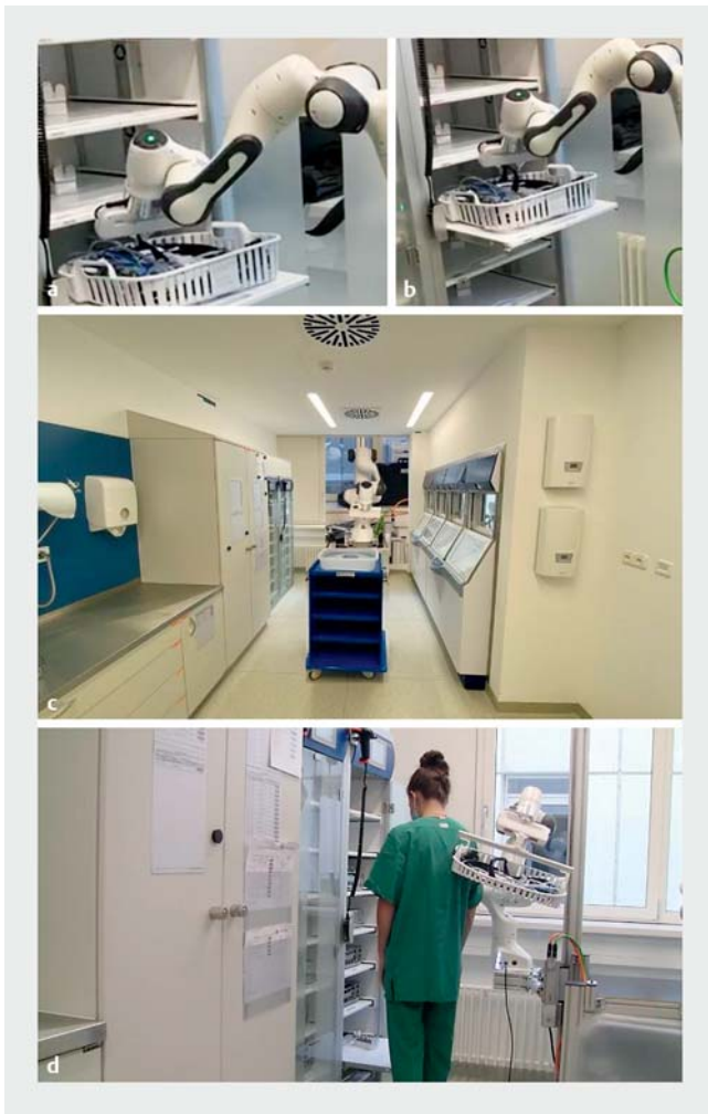
► Fig. 5 a Transfer of the endoscope from the storage cabinet b Opening of the lever to disconnect the individual venting lines. c Total view of the clean side with the autonomous trolley and the sterile plastic box for the endoscopic tray. d Collision detection of the system to avoid interference.
