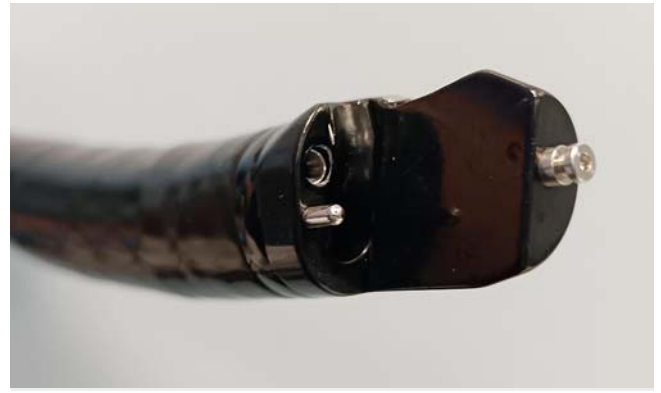
► Fig. 2 The image shows the distal portion of the endoscope, without wire and cap.
