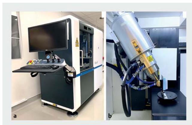
► Fig. 1 a Micro-CT scanner (Nikon Metrology NV, Leuven, Belgium). b Micro-CT scanning for whole-mount FFPE tissue block. CT, computed tomography; FFPE, formalin-fixed paraffin-embedded.
