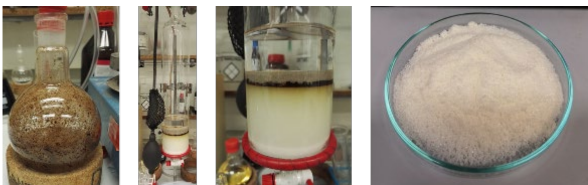
Figure S17. ( From left to right ) Obtained dimethyl 1,4-cubanedicarboxylate 1 after reaction + workup and dry-loaded compound on chromatography column and sample after purification.
