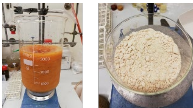
Figure S14. (Left) Refluxed solution poured in an ice-water bath (Right) obtained endo -2,4-dibromodicyclopentadiene-1,8-one 12 after drying under high-vacuum.
