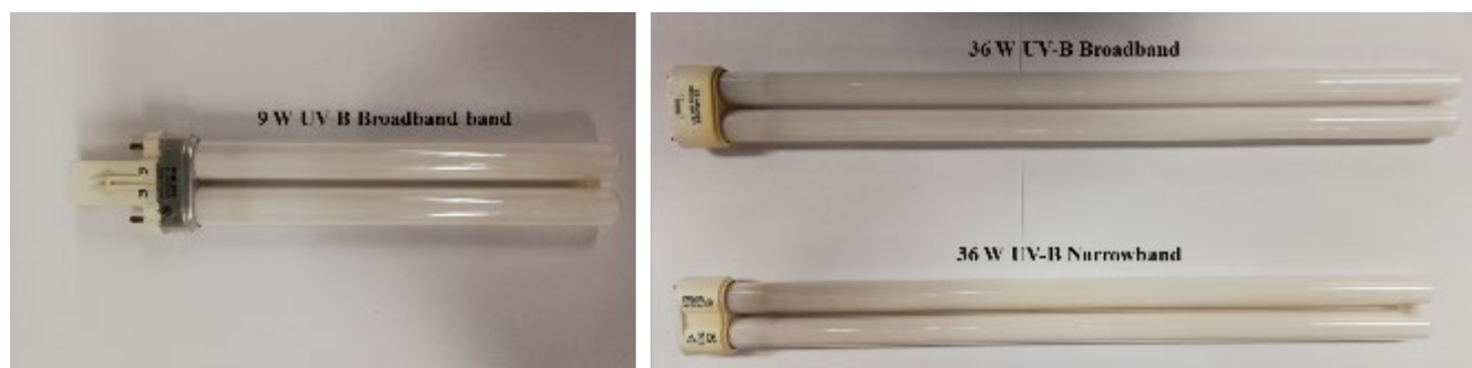
Figure S1. 9 W UVB-broadband and 36 W UVB–broadband and narrowband used for the [2+2] photocycloaddition.
