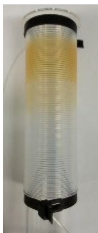
Figure S6. Irreversibly damaged FEP flow reactor after UV-C irradiation.
